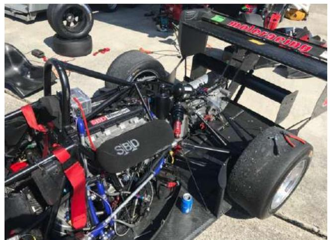
front rear balance changes event by event. And finally lesson 4. If your nose tells you there is a strange burning smell, don't ignore it and fob yourself off saying "it's a hot day – must be clutch or brakes", investigate! The fuel pressure sensor leg of the loom was touching an edge of carbon and cut through causing a small fire right next to the high-pressure fuel lines, but the car only ground to a halt and no permanent damage occurred.
